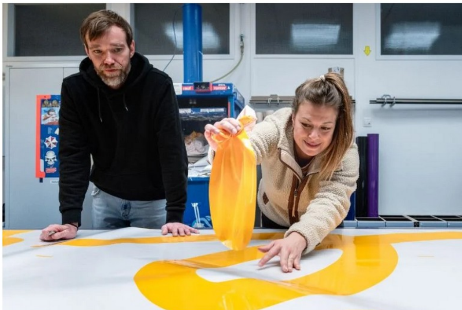
Since little to no solvent is required to remove decals, they generally produce less hazardous waste. Photo Credit: Lufthansa Technik
